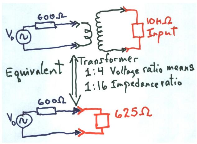
B) Inserting the transformer now makes the amplifier input appear to be easier to move – to use the mechanical analogy. If its impedance is transformed to  $625\Omega$ , how much power is now delivered to the amplifier input?
