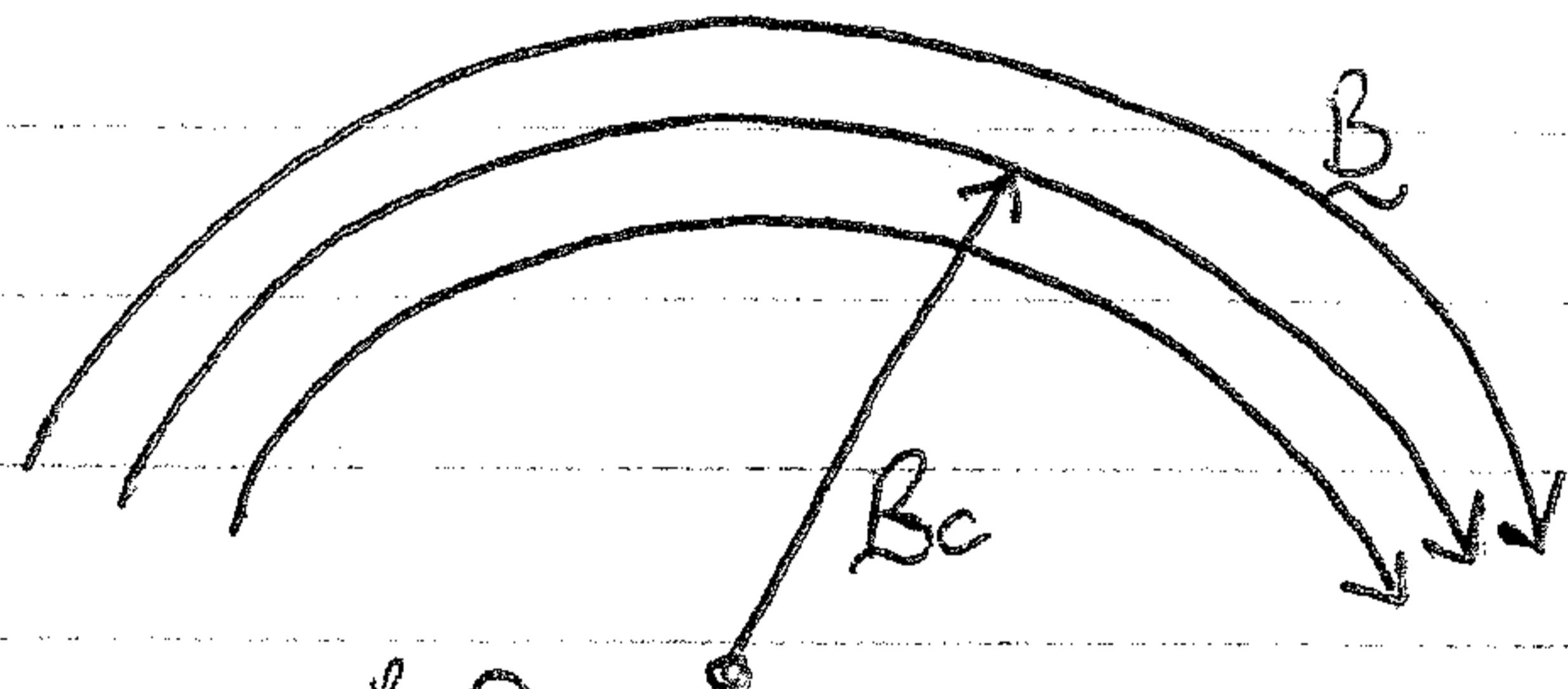
2. When field lines are curved, there is also typically a gradient in  $|B|$ , so both  $\nabla B$  and curvature drifts will be important.
