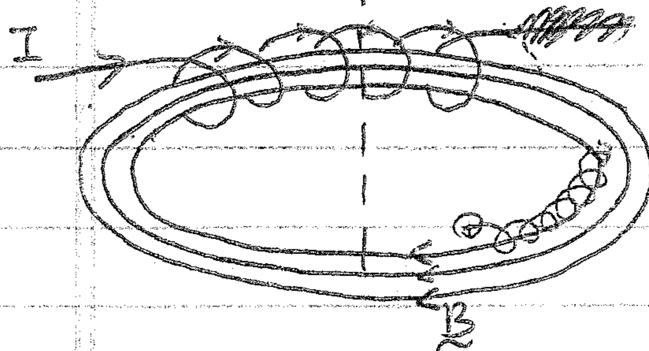
1. Toroidal Magnetic Field can be produced by winding a current-carrying wire around a torus.
