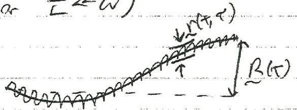
4.  $\underline{F}_{\text{pond}} = m \frac{d\underline{u}}{dt} = \frac{-q^2}{4\pi\epsilon_0 \omega^2} \nabla |\underline{E}_0|^2$
