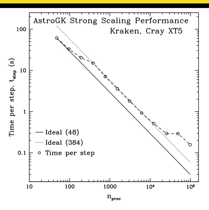
• Note: Kraken (Cray XT5) nodes have dual hex-core processors, so performance degrades as more cores/node are used due to memory bandwidth limitations
