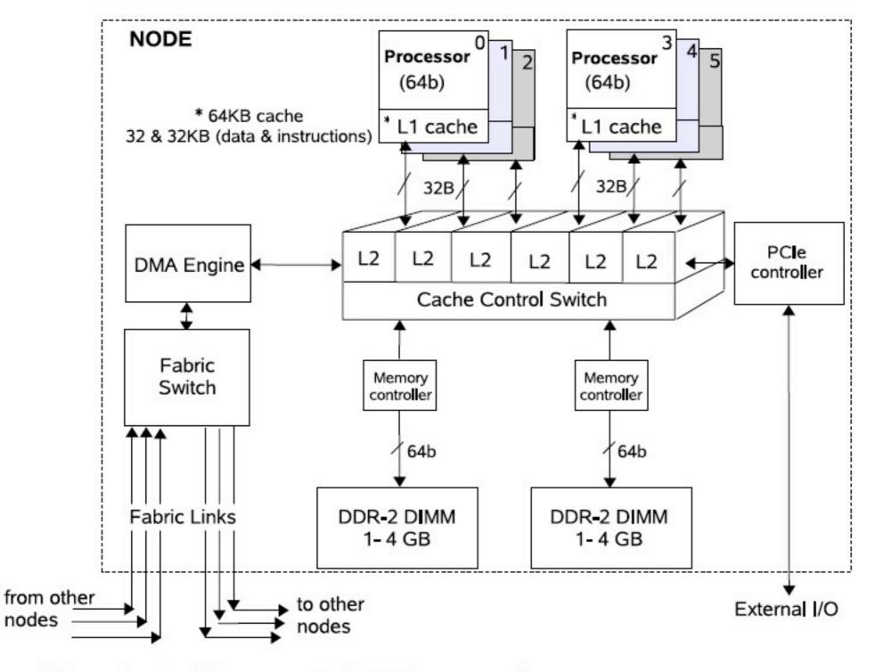
Figure 4. Architecture of the SiCortex node
