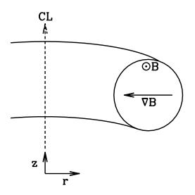
The lowest order motion is the Larmor motion about a toroidal magnetic field line which closes on itself. Consider the effect of drifts due to the topology of the magnetic field.
