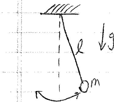
1. We wish to determine the dependence of the pendulum period  $T$  on the physical quantities  $l$ ,  $m$ , and  $g$ .
