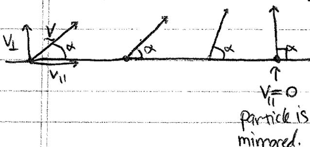
a.  $\mathcal{E} = \frac{1}{2} m v_{||}^2 + \mu B = \text{constant}$
