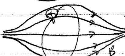
3<sup>rd</sup>! Magnetic Flux enclosed by drift orbit remains constant
