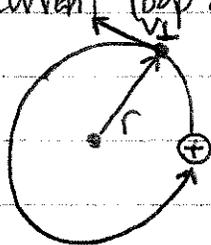
$$\mu = \frac{m v_{\perp}^2}{2B}$$
