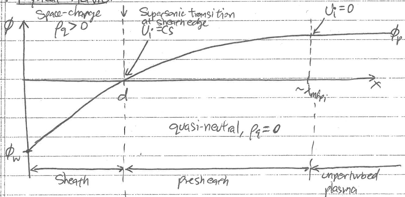
All plasma is causally disconnected from the sheath and wall.
