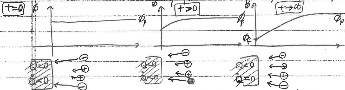
a) Since  $v_{fe} \gg v_i$ , electrons hit object more rapidly than ions  $\Rightarrow$  Object begins to charge negatively
