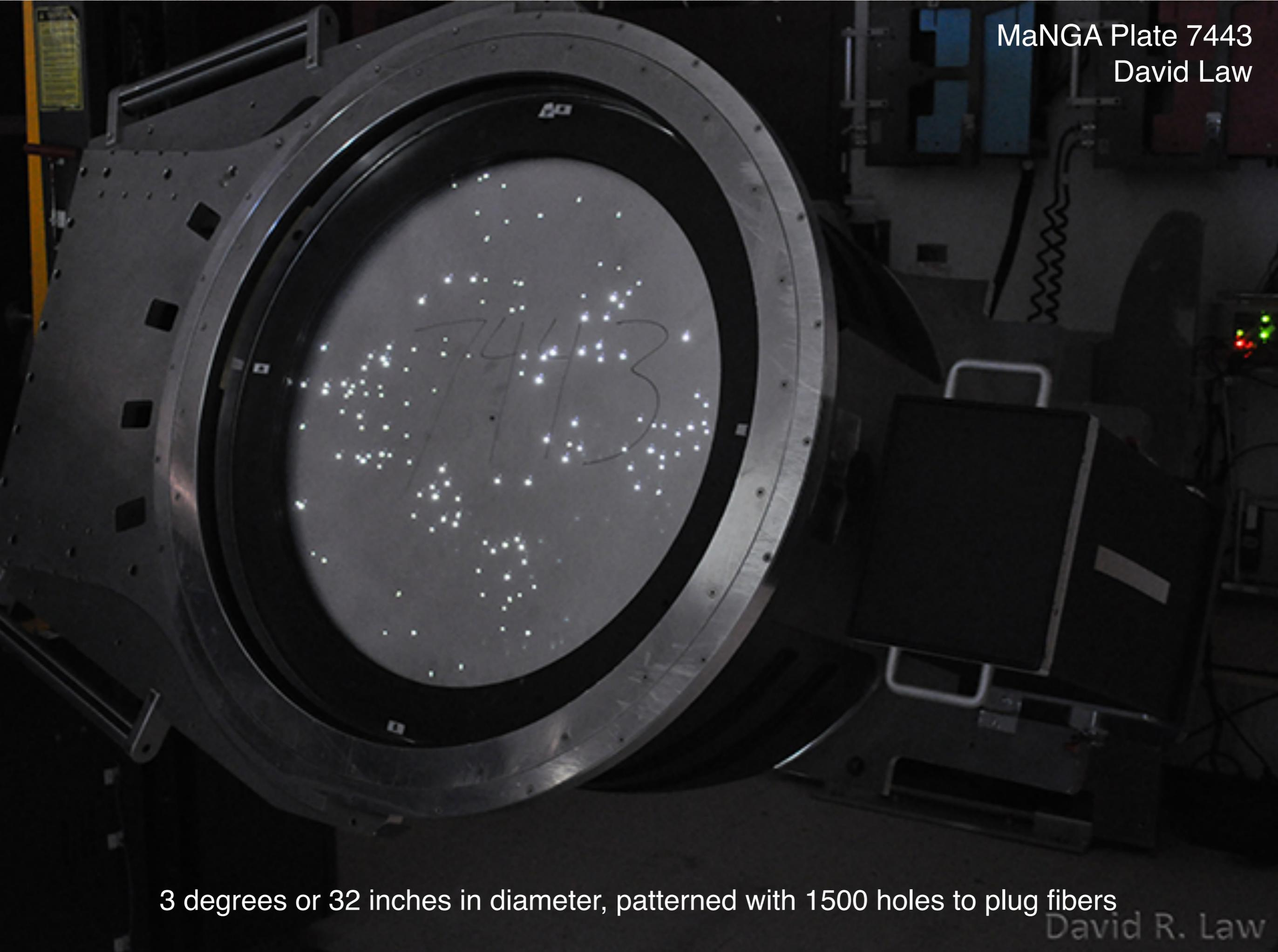
3 degrees or 32 inches in diameter, patterned with 1500 holes to plug fibers
