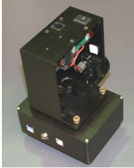
Figure 2: DSS-7 spectrograph connected to the ST-402 CCD camera.
