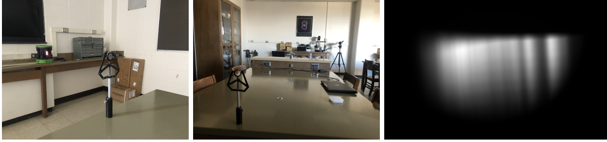
Figure 1: Spectrograph Setup 1. Left: Spectrum tube aligned with the SA-100 grating. Middle: The focuser (Orion refractor) placed at an angle to catch the 1st-order spectrum. Right: Example spectrum taken in this setup (note that the spectrum is truncated by the grating, meaning that the grating was placed too far from the focuser).
