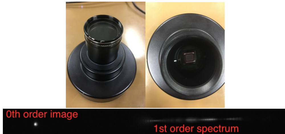
Figure 2: Spectrograph Setup 2. Top: the Orion camera attached with a Star Analyzer grating on the nosepiece. Bottom: example spectrum of an optical fiber mounted on the Nitrogen gas tube.
