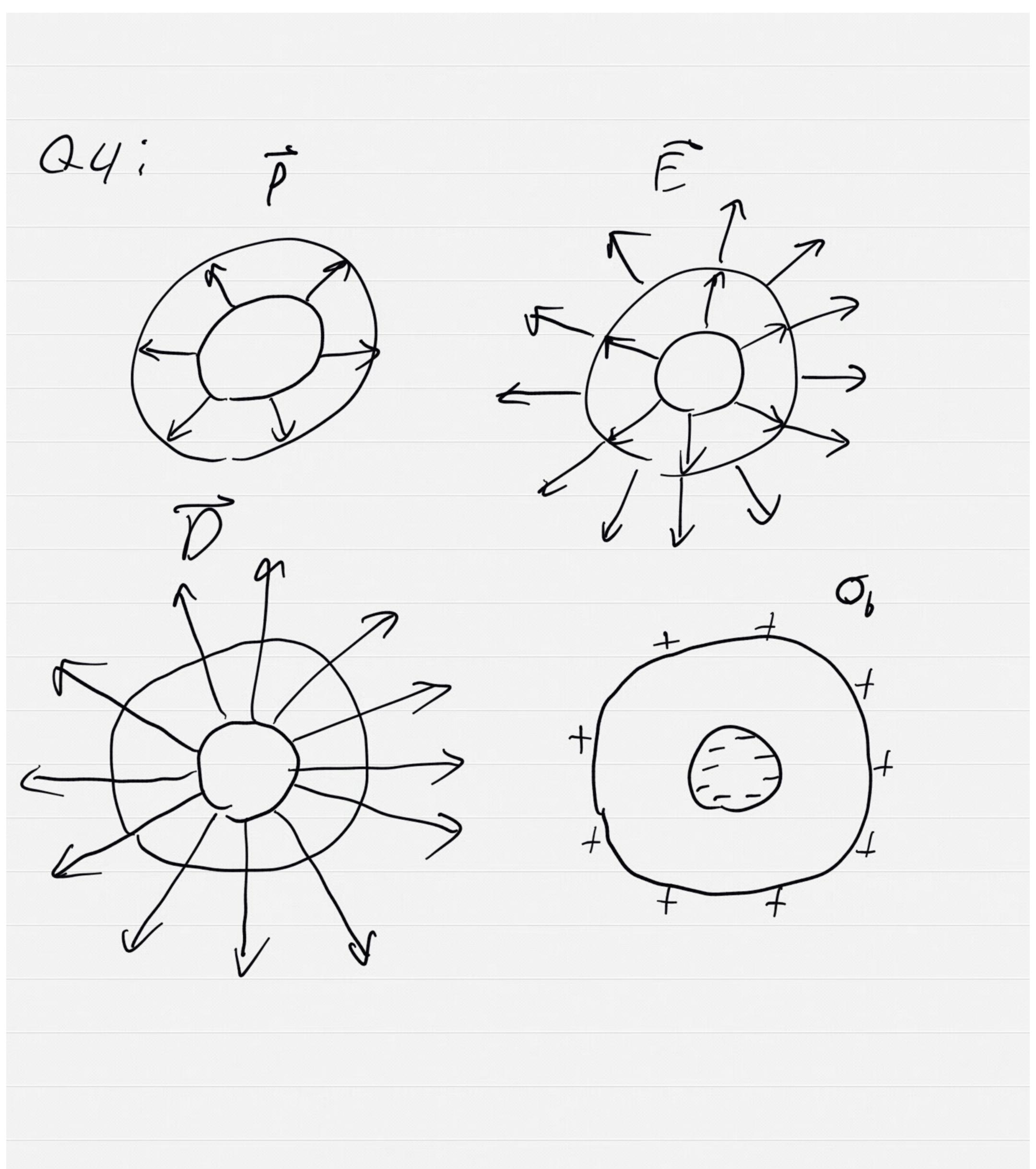
Consider a dielectric sphere embedded in an initially uniform external field. Sketch the resulting lines of polarization, electric field, and electric displacement.
