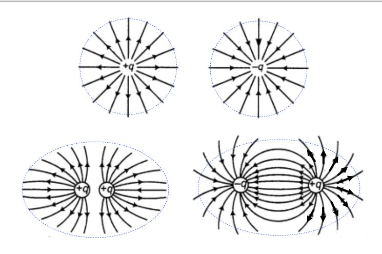
Charge enclosed -> electric field lines outward -> electric flux through surface
