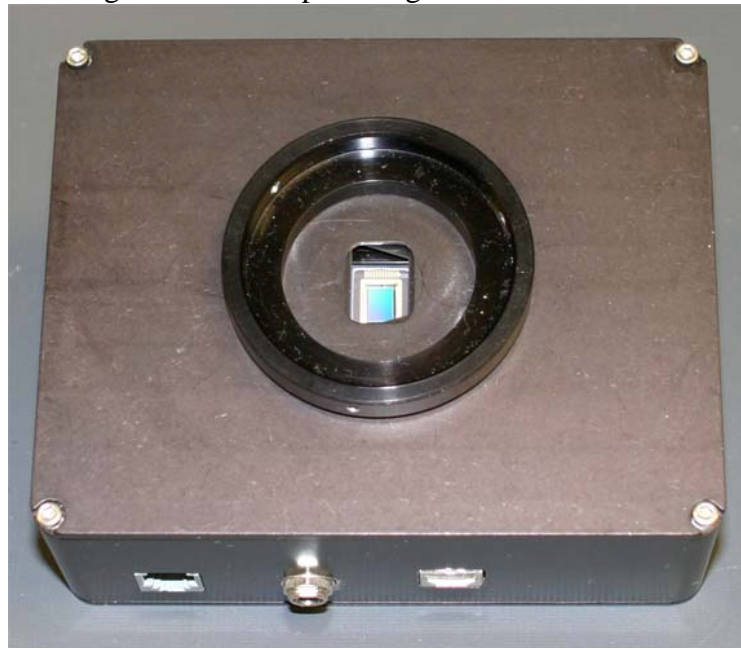
Figure Nine: Adapter Ring Mounted to ST-402
