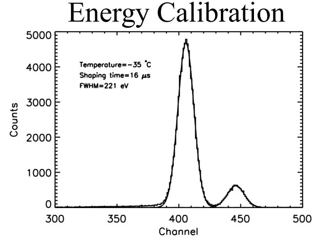
Shine a monochromatic X-ray beam on the detector, then measure the response. Use several different energies to find energy versus channel conversion. Also, need to know shape of response and efficiency at each energy.
