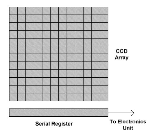
At regular intervals (the frame time), the contents of the active region is transferred to the frame store, then the charge in each pixel is measured using an A/D converter. We get out a digital value (the pulse height amplitude = PHA) for each pixel representing the charge in that pixel.
