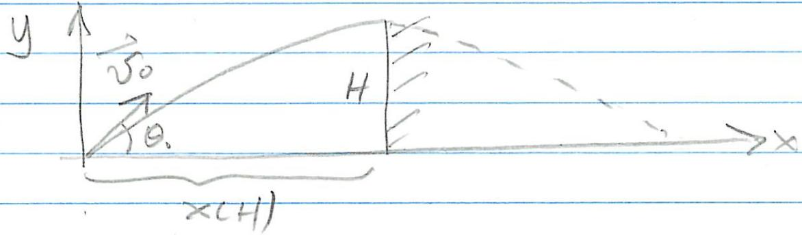
The firehose should be placed so that the highest part of the building is at the maximum vertical point of the trajectory,  $y_{\max} = H$
