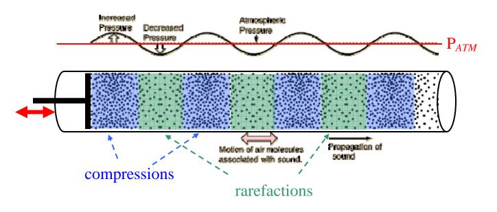
A harmonic sound wave consists of a series of high density (compressions) and low density (rarefactions) regions that propagate down the tube.
