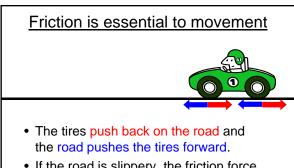
• If the road is slippery, the friction force between the tires and road is reduced, and the car does not move..
