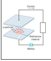
Smoke detectors have a radioactive alpha emitting source. The alpha particles ionize the air in the detector creating a current. If smoke particles enter the detector they can interfere with the current causing it to drop, which sets off the alarm.
