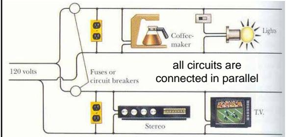
all circuits are connected in parallel
