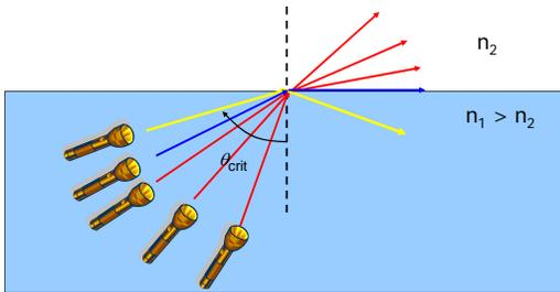
When,  $n_1 > n_2$  and the incident angle is greater than a certain value ( $\theta_{crit}$ ), the refracted ray disappears, and the incident ray is totally reflected back into the medium.
