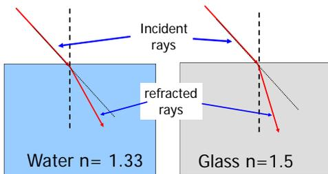
The refracted ray is bent more in the glass
