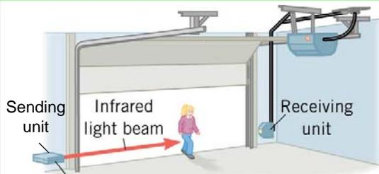
The child interrupts the beam, stopping the current, which causes the motor to stop.
