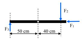
Solution- The net torque is the sum of thetorques produced by F<sub>1</sub>, F<sub>2</sub>, and F<sub>3</sub>. Since the line of action of F<sub>3</sub> passes through the axis, it produces no torque. Both F<sub>2</sub> and F<sub>3</sub> produce torques that both cause clockwise rotation, so their net effect is additive.
