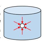
to that surface. The water on top of the object pushes down on it and the water below the object pushes up on it, etc. Since the object is very small, the value of the pressure is roughly the same on all of its sides.
