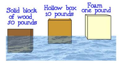
Note that in any situation, if the maximum possible buoyant force is less than the weight of an object, the object will sink to the bottom
