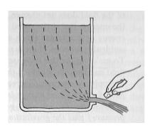
the opening. The pressure in the moving liquid is reduced. The faster the liquid moves, the lesser the pressure in that liquid.
