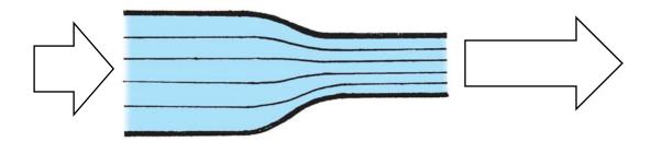
necessarily, since all the fluid entering the left side must exit the right side, the streamlines are bunched together in the constriction. Recall that the continuity principle requires that the fluid must flow faster in the constricted region, then, according to Bernoulli, the pressure of the fluid in the constricted region must be lower because the fluid speed is higher there. **So we can associate the bunching of the streamlines with higher speed flow and therefore lower fluid pressure.**
