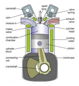
the molecules in the cylinder to expand very quickly causing the piston to move quickly. The
