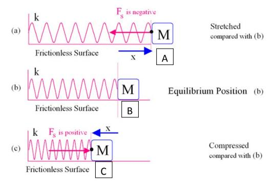
stretched nor compressed. If the mass is pulled to the right as in (a) above, the spring pulls it back to equilibrium. The mass continues moving to the left, past its equilibrium position as in (c), and now compresses the spring. The spring then pushes it back to the right. **The amplitude of oscillation is the maximum distance (A) that the object is initially displaced from its equilibrium position.** The mass then oscillates back and forth from x = +A to x = -A.
