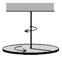
As it continues to rotate, the wire now becomes twisted in the opposite direction, thus providing a mechanism to maintain an alternating clockwise and counterclockwise rotation.
