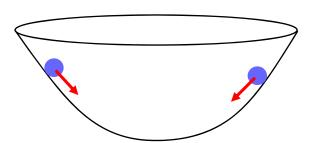
left, and when it is on the right side, gravity pulls it to the right. In either case gravity acts as a force to "restore" the marble to its equilibrium position at the bottom of the bowl. Gravity is the restoring force for the pendulum and the spring provides the restoring force for the mass/spring system.
