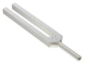
motion of the prongs is too small to see, however, the vibration of a prongs causes the air surrounding them to vibrate, and the vibration in the air travels away as a sound wave which we hear when it causes our eardrums to vibrate. Tuning forks are designed to produce a sound wave with a pure pitch (frequency). The tuning fork shown produces the musical note C at 512 vibrations per second.
