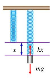
**Example 20-3:** A mass of m = 2 kg is hung vertically from a spring having a spring constant k = 1000 N/m. By how much will be spring be stretched from its relaxed position?
