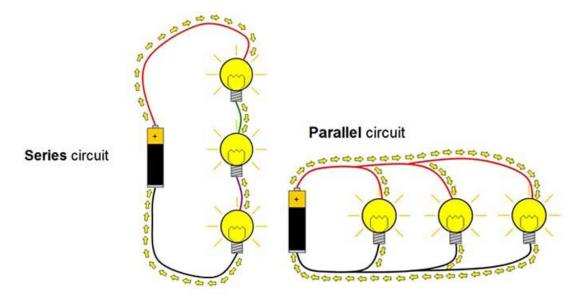
The circuit on the left is called a **series circuit**, and the circuit on the right is called a **parallel circuit**. The arrows show the current flow.
