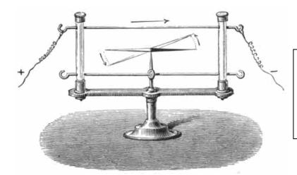
Oersted's apparatus showing that a current in a wire caused a nearby compass needle to rotate. This established the principle of electromagnets.
