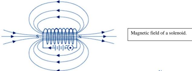
A **simple electromagnet** can be made using a nail with wire wrapped around it and a battery to drive current in the wires. When current is applied to the coil surrounding the nail, the nail becomes magnetized and a stronger magnetic field is produced than the field of the coil alone. The magnetization of the nail is not permanent and will diminish quickly after the current in the coil is turned off.
