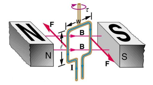
When this loop is attached to a shaft, the device is an **electric motor**, which converts electrical energy into mechanical energy. Some additional applications of magnetic forces are illustrated **on slides 19, 24, and 25.**
