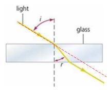
through a plane slab of glass as shown on the left side. In this case the exiting light ray will be
