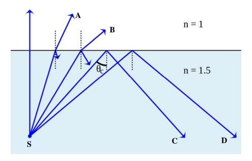
Total internal reflection is the process used in fiber optic communications. Light is sent down
