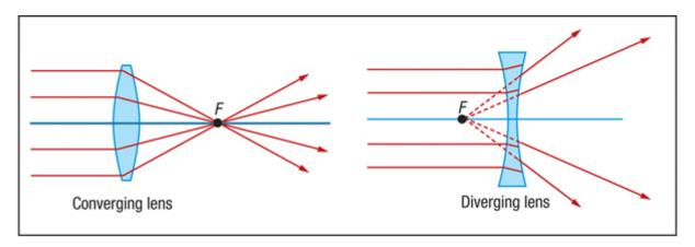
rays is shown below. A converging lens causes parallel light rays to converge to a focal point F on the right side. A diverging lens causes parallel rays to diverge or spread out as if they originated at the focal point F on the left side
