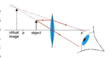
VIRTUAL, UPRIGHT, and ENLARGED. This is the configuration of a magnifying lens.
