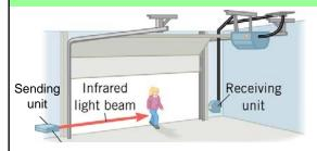
The child interrupts the beam, stopping the current, which causes the motor to stop.
