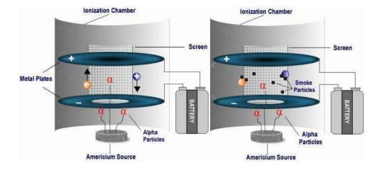
material that emits alpha particles. The alpha particles knock electrons off of air molecules which then flow to a positive plate creating a small current that is detected by an electronic circuit. When smoke particles enter the region between the two plates some of the ions attach to them, and this disrupts the flow of current. When the electronic circuit senses a drop in current it sets
