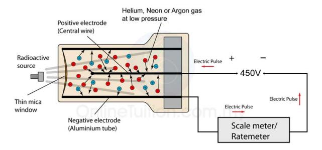
ionization of the inert gas atoms by alpha, beta, or gamma particles that enter the thin mica window. When one of these particles enters the tube, it is energetic enough to knock electrons out of the inert gas atoms (ionization). The liberated electrons migrate to the positive center wire acquiring energy as they move toward it. As a result, the liberated electrons can ionize more atoms. Liberating even more electrons which can also ionize. As a result, an avalanche of
