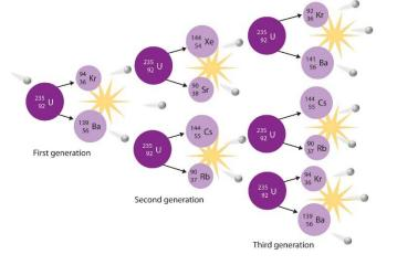
reaction is allowed to proceed in a **controlled** manner, this process can be used in a nuclear reactor to make electricity. The first controlled nuclear chain reaction was demonstrated by **Enrico Fermi** in 1942 in a laboratory under the stands of Stagg Field at the University of Chicago. If the chain reaction occurs in an **uncontrolled** manner, there is a sudden and catastrophic release of the nuclear energy --- this is a nuclear bomb.
