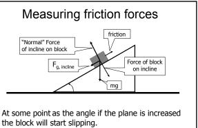
At this point, the friction force and gravity are equal.
