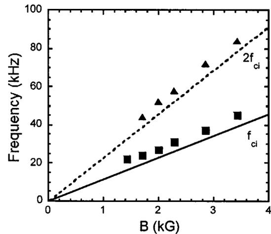
FIG. 5. Dependence of the frequency of the fundamental and first harmonic EIC mode on magnetic field strength for a collector located in the region of transverse shear ( $102^\circ$ ). Solid line:  $f_{ci}$ ; dashed line:  $2f_{ci}$ .
