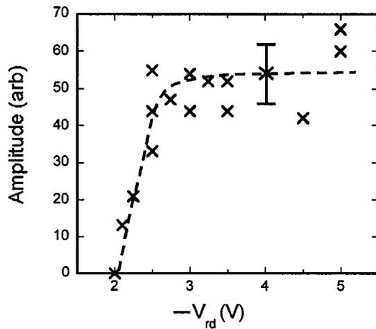
FIG. 4. Amplitude of EIC instability for the collector at  $\theta=102^\circ$  versus the negative ring+disk bias voltage. Same conditions as in Fig. 3.
