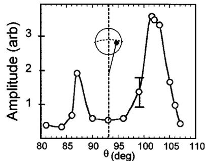
FIG. 3. Amplitude of the EIC instability ( $f = 39$  kHz) as a function of the radial position ( $\theta$ ) of the collector in the plasma column. The center of the column corresponds to roughly  $\theta = 93^\circ$  (dashed line) and the edges of the disk at  $\theta = 87^\circ$  and  $\theta = 102^\circ$ . Here  $B = 2800$  G,  $\rho_i = 2$  mm,  $r_c = 1.5$  mm,  $V_c = -0.4$  V, and  $V_{rd} = -5$  V. The baseline corresponds to the background noise level.
