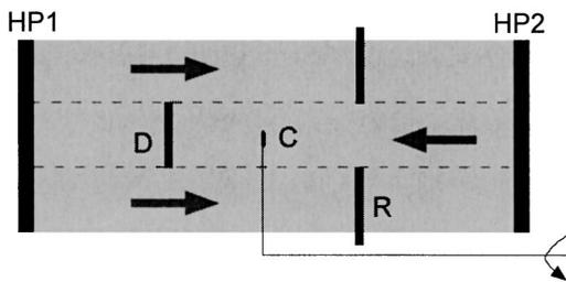
FIG. 1. Schematic of the experimental setup. Cesium plasma is produced by contact ionization of Cs atoms from atomic beam ovens (not shown) on the two hot plates (HP1, HP2). The ring+disk configuration (R,D) is used to produce magnetic field-aligned ion flow with a fluid velocity gradient in the direction perpendicular to **B**. A small disk collector (C) is used to drive electron current along the magnetic field lines.
