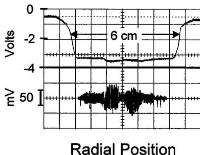
FIG. 2. Upper trace: radial profile of the floating potential of a Langmuir probe. Lower trace: radial profile of low frequency oscillations driven by transverse shear in the parallel ion flow. The positions of peak amplitude correspond to the regions of largest shear.
