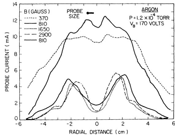
Fig. 6. Radial profiles of electron saturation current ( $\sim$  electron density) for various magnetic field strengths in argon.
