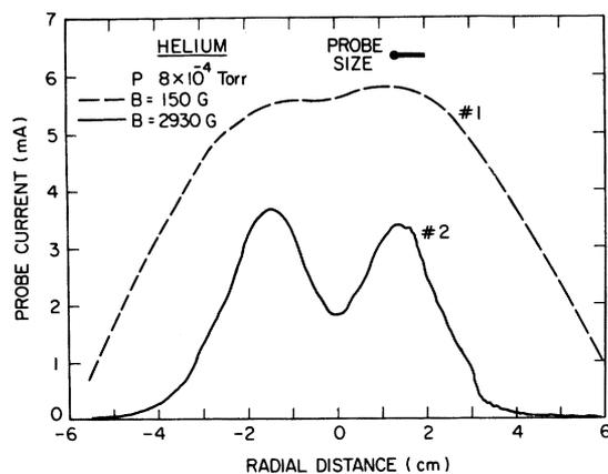
Fig. 7. Radial profiles of electron saturation current ( $\sim$  electron density) for  $B = 150$  G and  $B = 2930$  G in helium.
