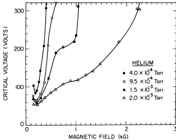
Fig. 4. Critical voltages for upgoing transitions versus magnetic field strength for helium plasmas at various pressures.
