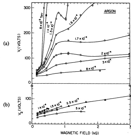
Fig. 3. Critical voltages for (a) upgoing transitions, and (b) downgoing transitions, versus magnetic field strength for argon plasmas at various pressures.
