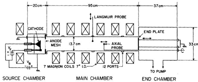
Fig. 1. Schematic diagram of plasma discharge device.
