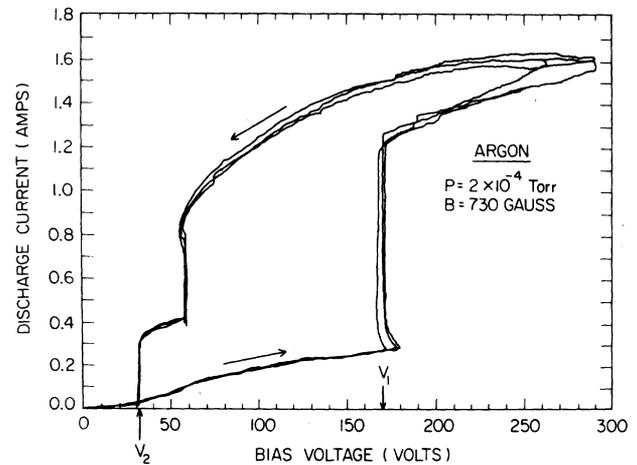
Fig. 2. Discharge current  $I_D$  versus bias voltage  $V_B$  at fixed magnetic field strength showing sudden jumps and hysteresis.
