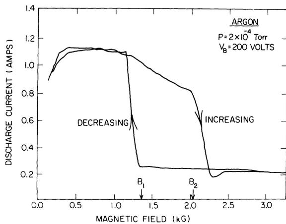
Fig. 5. Discharge current versus magnetic field strength showing sudden jumps and hysteresis. Note that in this case the magnetic field strength was changed slightly as the x-y recorder was responding to the rapidly changing current.
