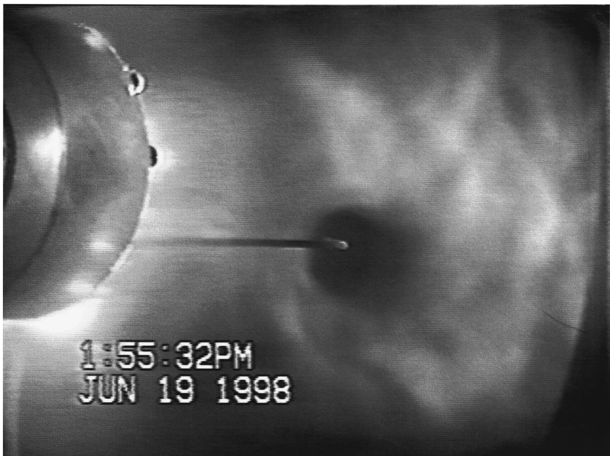
FIG. 2. Single frame video image of the “object” at rest in the dusty plasma.
