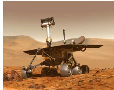
The Mars Exploration Rovers (MER) are mobile, geological laboratories sent to see if Martian rocks are lava flows (e.g. basalts) or minerals formed in the presence of water.
