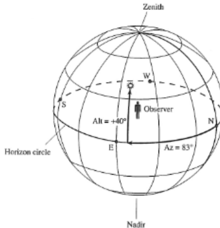
FIGURE 1.3 Altitude (Alt) and azimuth (Az) of a point on the celestial sphere, as seen by an observer on Earth.
