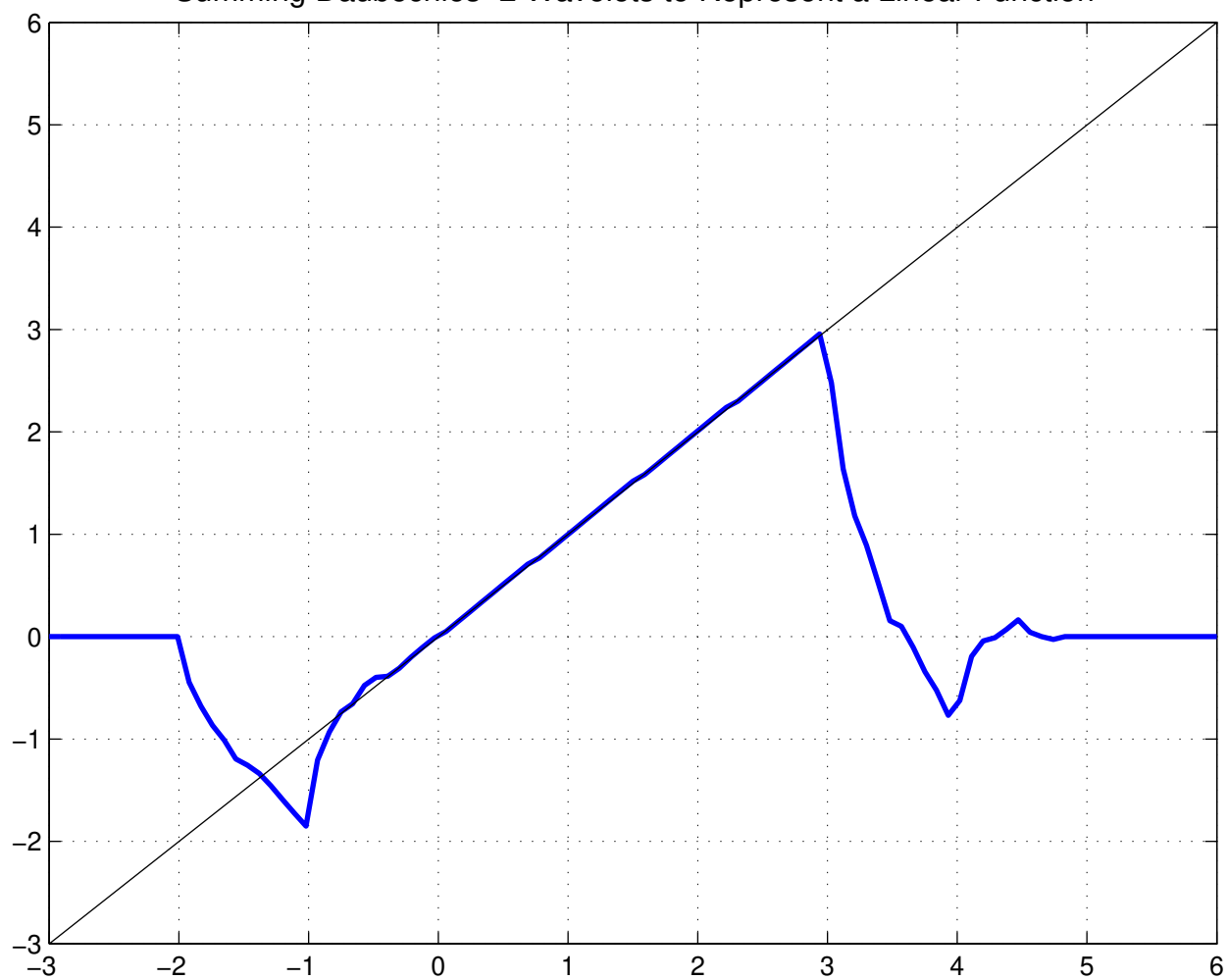
Summing Daubechies-2 Wavelets to Represent a Linear Function
