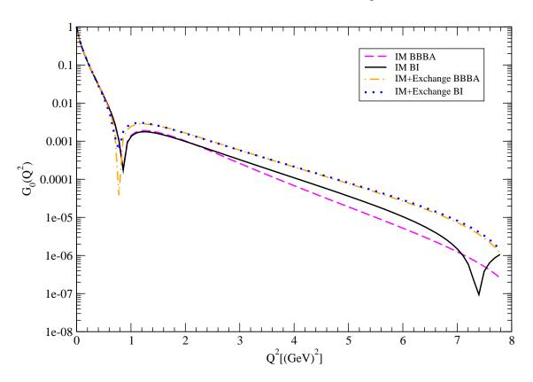
FIG. 5: Deuteron form factor  $G_0(Q^2)$  with and without exchange current
