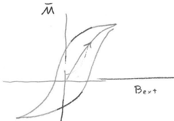
In this case the magnetization is a multivalued function of the applied field.
