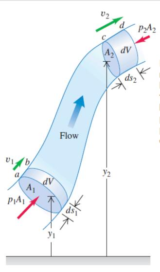
Deriving Bernoulli's equation. The net work done on a fluid element by the pressure of the surrounding fluid equals the change in the kinetic energy plus the change in the gravitational potential energy.
