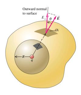
The electric flux thru any <u>closed surface</u> S is a constant  $(1/\epsilon_0)$  times the <u>net charge enclosed</u> by S.
