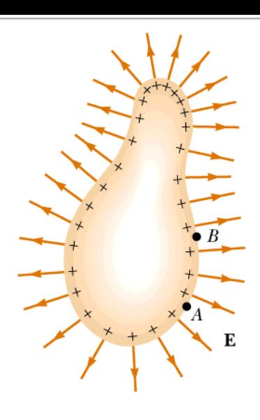
anductors = 0 since 1=0 so V = constant in conductor - This means the surface of a conductor is an equipotential, - E = - TV must be perpendicular to equipotentials - Sa É perpendicular to surface of canductor
