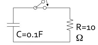
Answer:  $1/e^2 A = 0.14A$ . The time constant for this circuit is  $RC=(10\Omega)(0.10F) = 1.0$  sec. So at time t=2.0 sec, two time constants have passed. After one time constant, the voltage, charge, and current have all decreased by a factor of e. After two time constants, everything has fallen by  $e^2$ . The initial current is 1A. So after two time constants, the current is  $1/e^2 A = 0.135A$ .
