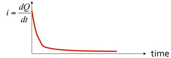
Energy Pissipation Charging Ceptel = SIV St = 5° V6 - V, e - + RC St = \frac{V\_0^2}{R}. - RC e^{-tR(\frac{100}{9})}  $= CV_b^2$ Uc = 1200/c = 1200/2 - Half of power dissipated in resistor while charging, half goes to capacitor
