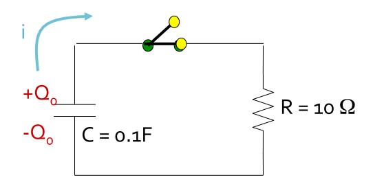
Close the switch at t=o, then current i starts to flow.
