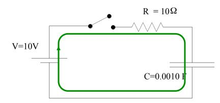
Before switch closed i=0, and charge on capacitor Q=0.
