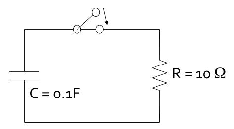
Initially one has  $+Q_o$  and  $-Q_o$  on the Capacitor plates. Thus, the initial Voltage on the Capacitor  $V_o = Q_o/C$ . What do you think happens when the switch is closed?
