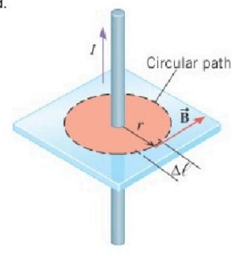
Amperes Law: Thick Wire same solution as thin wire Fuside  $\int \vec{D} \cdot \vec{J} \vec{e} = B(r) \cdot 27 r$ I enc = SJ-dF = J-A = J-dF = J-A = I · Tr2/AR2 = Ir/22 B(V) = m. I 1/2 - /2#r po In 2002 r 2R B(1)
