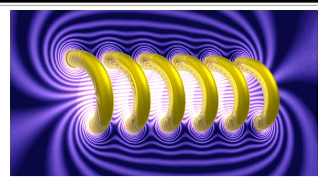
A single wire tightly coiled up into loops. Since it is a single wire, the current magnitude is the same in all parts of the coil. Solehoid 5+acked More tightly spaced I stronger axial field in center (and heaven outsite)
