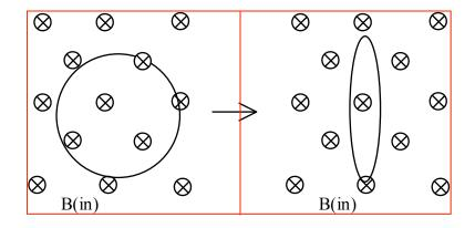
Answer: Clockwise. The flux into the page is *decreasing* as the loop area decreases. To fight the decrease, we want the induced B to *add* to the original B. By the right hand rule (version II), a clockwise induced current will make an induced B into the page, adding to the original B.
